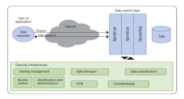
Figure 2-10: Logical Deployment of DCSM (Bilger et al., 2006)
