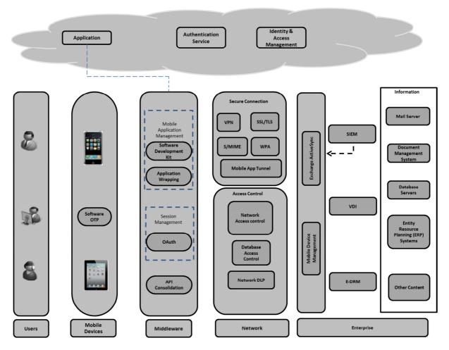
Figure 5-4: Derived Mobile Security Architecture Model
