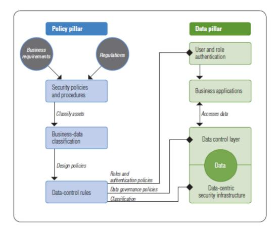
Figure 2-9: The Components of DCSM (Bilger et al., 2006).
